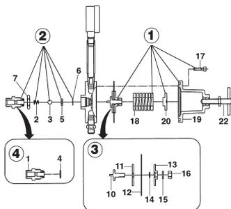
1. Fully loosen handle set (22), and remove bolts with hex.hole (17), diaphragm cap (19), spring holder (20), adjusting spring (18) and diaphragm section.
